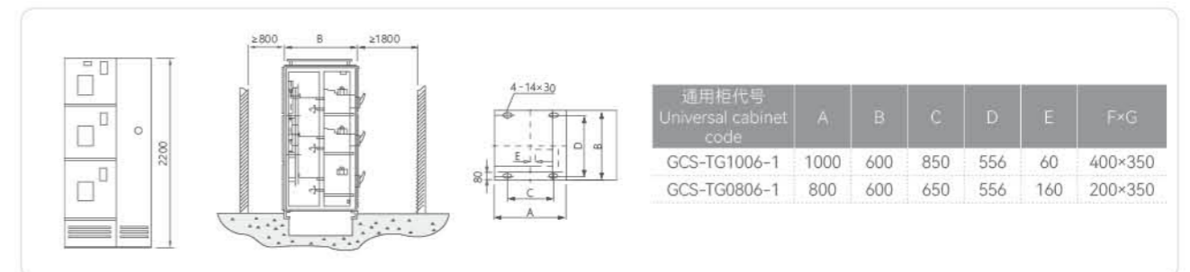
图 3、MCC 柜安装示意图 Figure 3. Installation diagram of MCC cabinet
