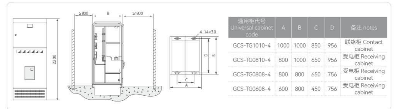
图 2、PC 柜安装示意图 Figure 2. Installation diagram of PC cabinet
